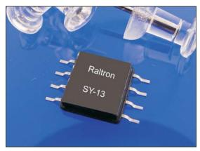
Raltron's SY13 Frequency and Phase Detector is provided in an 8-lead SMT package with 0.1 inch lead spacing.
